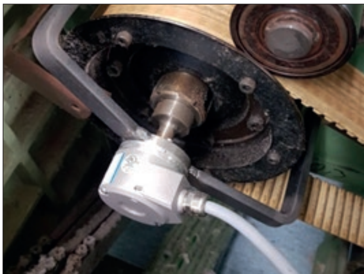
Example of encoder installed on a weaving machine
