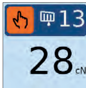
Manual (MAN) mode. Orange icon, with brake holder position in number of steps
