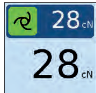
Automatic (AUTO) mode. Green icon, with target or reference tension ATC has to maintain.
